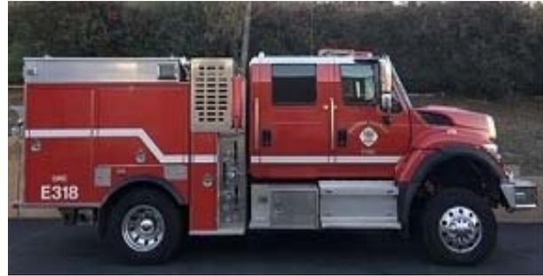
**Project Description:** The Type III engine carries hose, water and a skid mounted pump, giving the apparatus the capability to pump while driving. The unit’s primary objective is for off-road wildland firefighting and rescue operations. These engines are smaller by design to maneuver on truck trails and rural areas.
